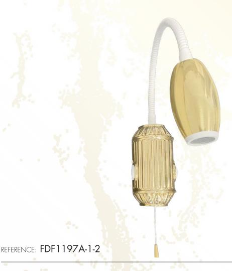
This reading lamp is like a built-in mechanism, so you can install it in a standard built-in box next to the headboard. You can move it, to direct the light when you need it. It incorporates a 2.6W direct Bi-Pin G9 LED LAMP at 230V and a color temperature of 2700°K, to create a cozy atmosphere. Available with pull cord switch or toggle switch.
