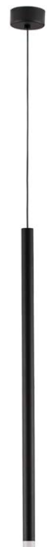
DANDIA - 9540200 Black Aluminum LED 6 Watt 220-240 Volt 367 lm 3000K IP20 D: 8 H: 150 cm 8 3.5 72 150 2.8 LED WARM WHITE DRIVER INCL.
