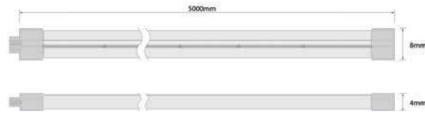
-RUBBER LED STRIP 6W/M IP67
