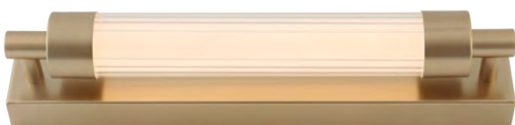
2. KALIA | Wall lamp WL32187/8W/GD 1 x 8W MAX LED 711LM 3000K metal | gold body glass shade
